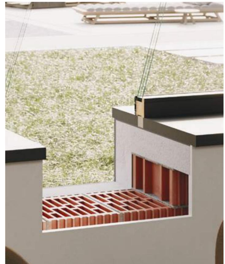
Detail of the bottom transom with thermal break of the fixed Blend window inserted in a niche that allows for an internal window sill.
