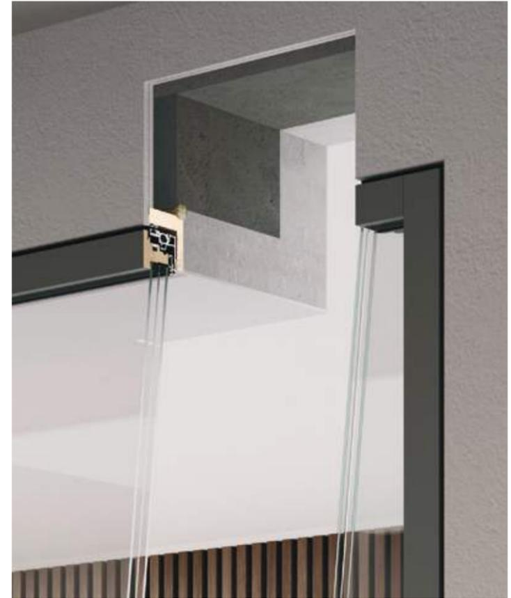
**Detail of the subframe and top rail of a Compact double-leaf French window in the presence of masonry, external insulation and plasterboard counterwall.**
