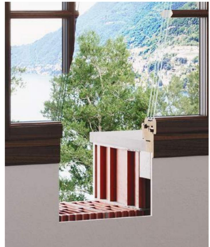
Detail of the bottom transom node with thermal break of a single-sash X-trim window inserted in masonry with marble sill and internal plasterboard counterwall.
